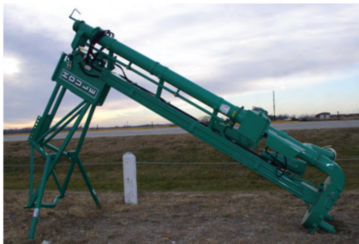
Figure 9. Agitation pump for liquid manure storage pits or tanks. This style of pump can be powered by electric motor or tractor PTO.
