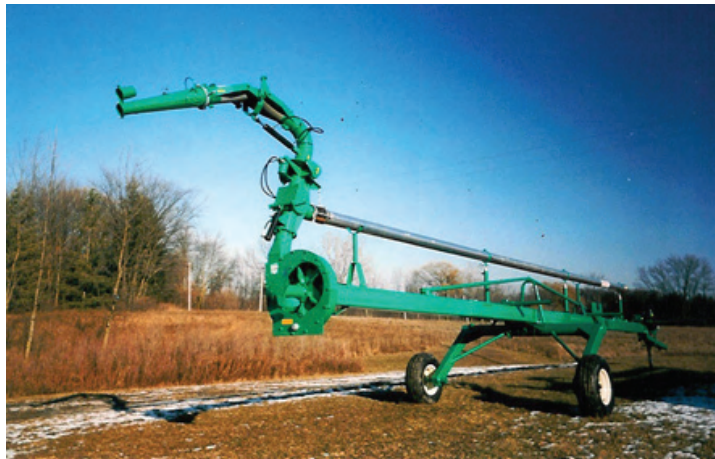
Figure 8. Large liquid manure agitation pump used to keep solids in suspension during application via ground applicator or center pivot.
