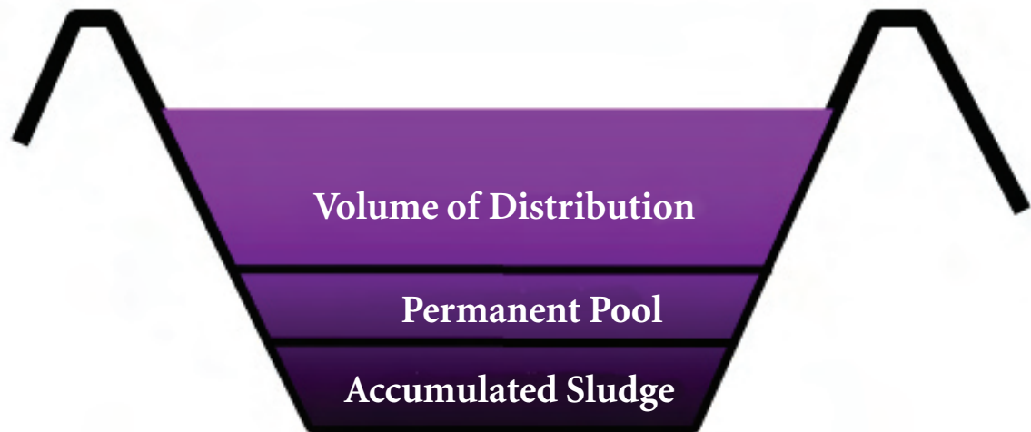
Figure 5. Stratification and design allocation of storage capacity in an anaerobic lagoon.
